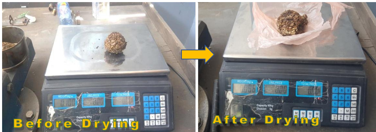
Figure 5-8: Measurement of mass of a sample briquette before and after drying
