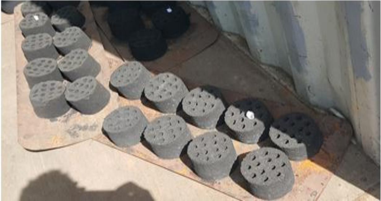
Figure 1-1: The open sun honeycomb charcoal saw dust briquette drying process [23]
