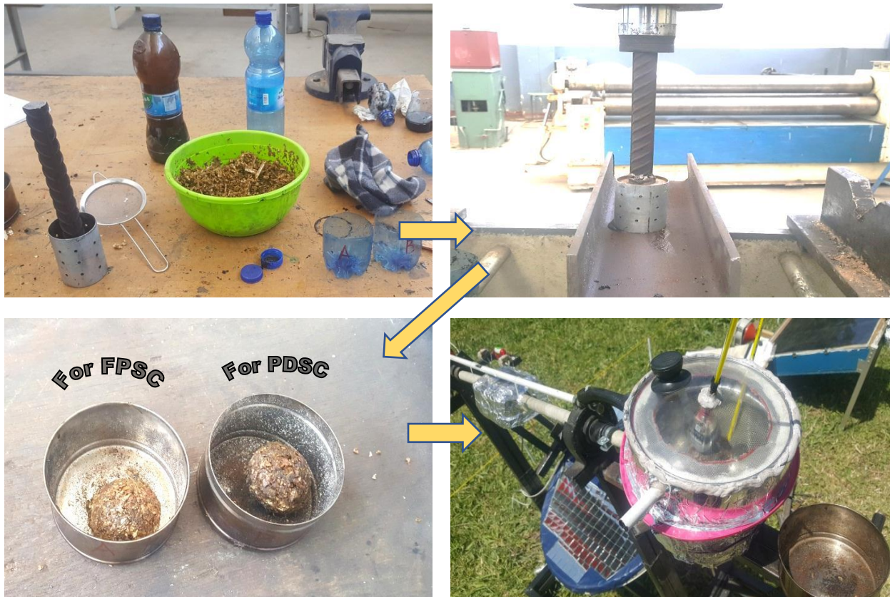
Figure 5-6: Process of saw dust briquette molding for preparing to drying experiment
