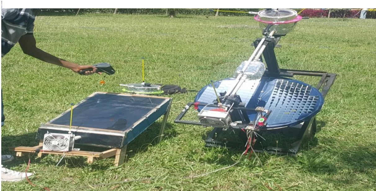
Figure 5-5: PDSC and FPSC Experimental dryers on the Testing process
