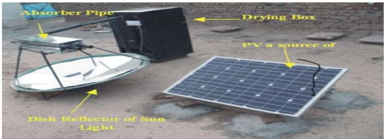
Figure 2-6: The dish type solar air heater for dryer [22]
