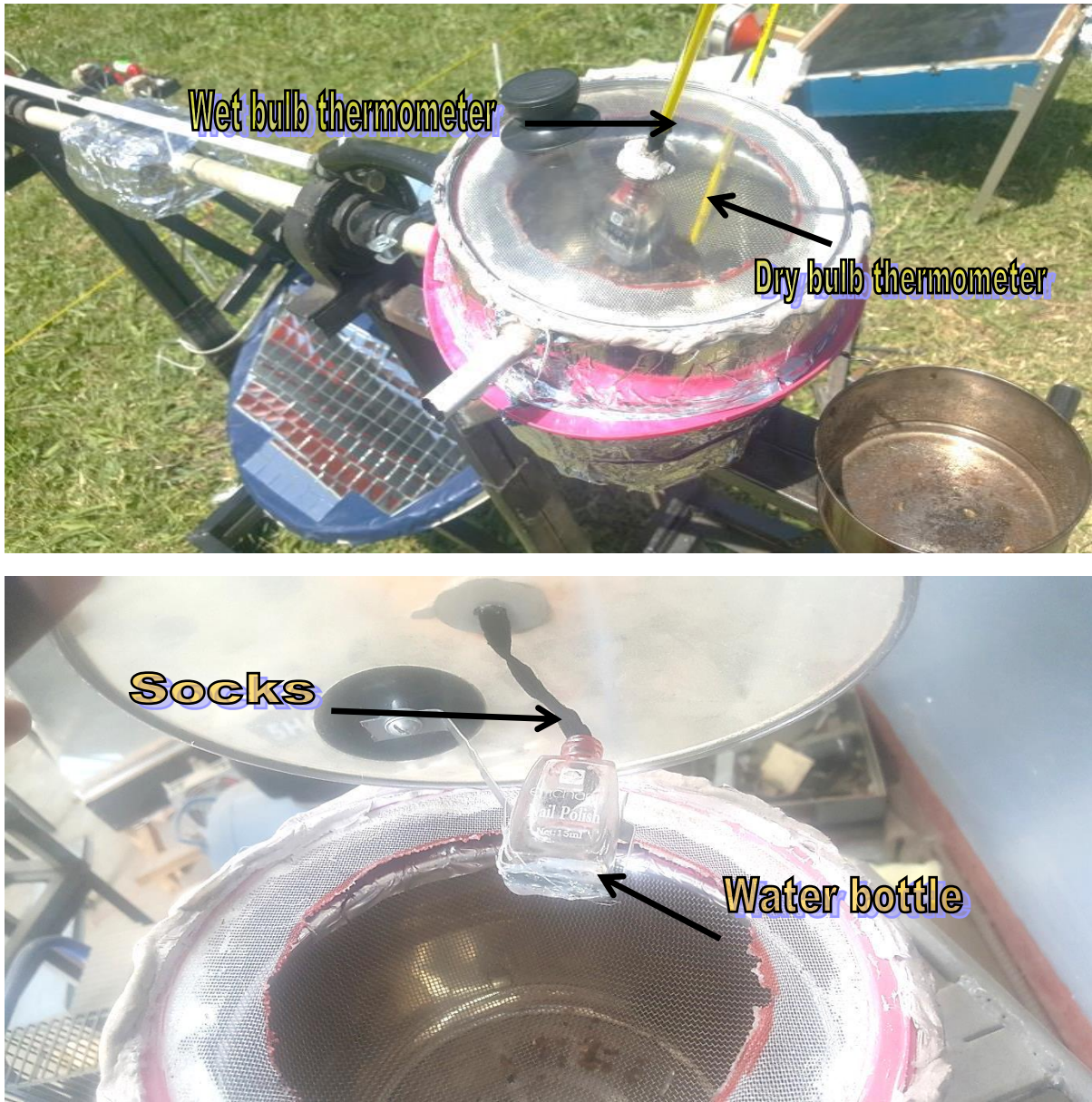
Figure 5-12: wet and dry bulb Thermometer on the drying chamber
