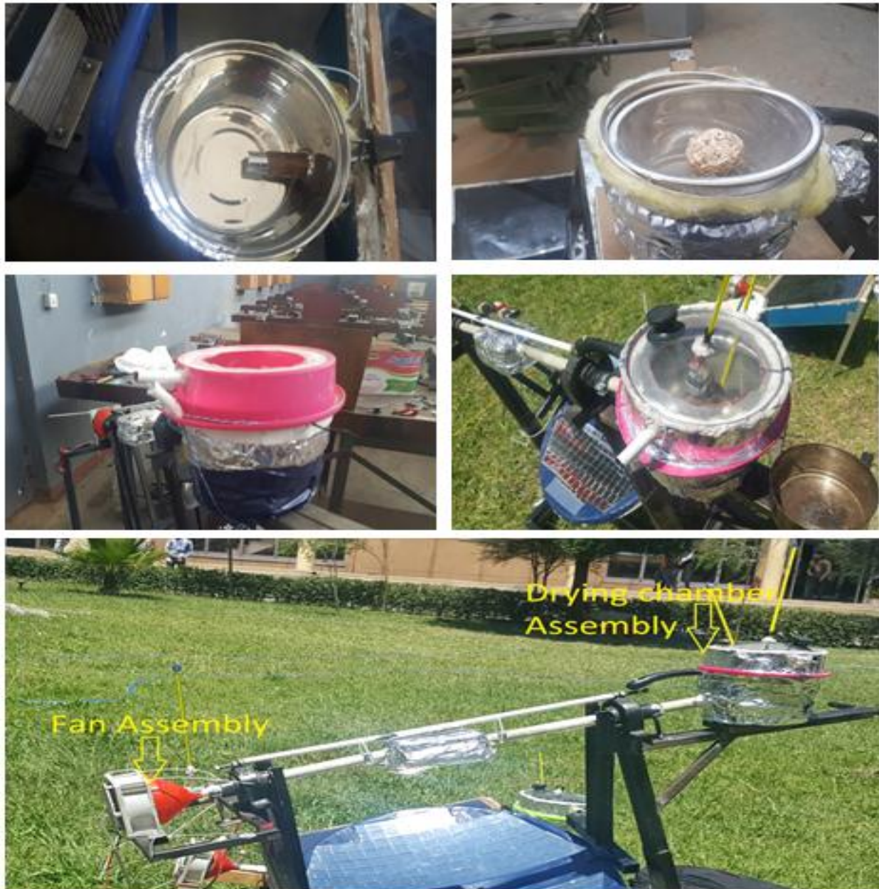
Figure 4-12: Fan and drying chamber assembly attached with the PDR support
