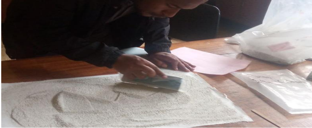
Figure 3.3 shows the removal of the ferromagnetic mineral before electromagnetic separation test for each size fraction
