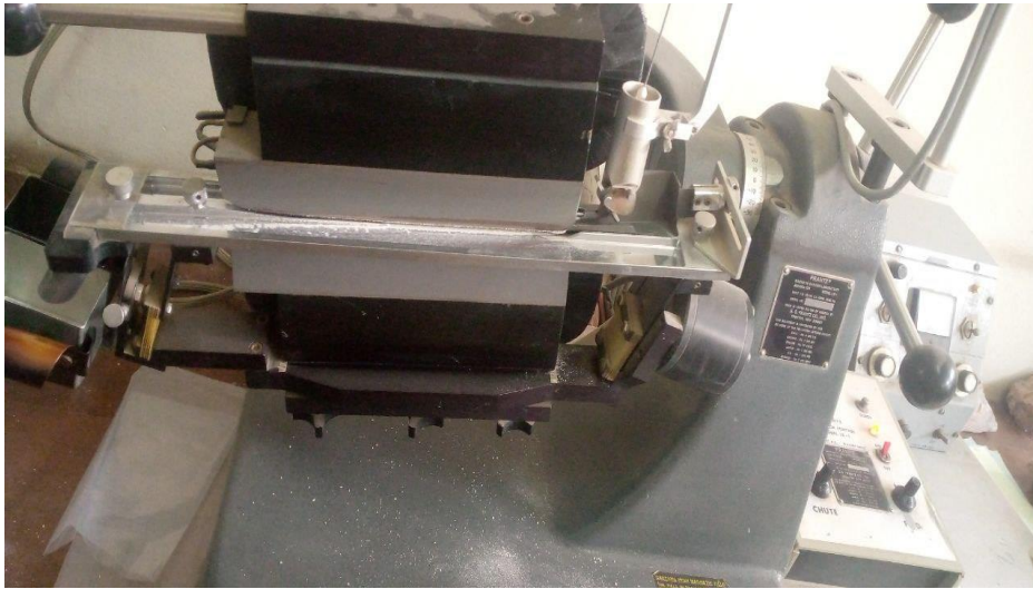
Figure 3.5. The electromagnetic separator tilted to angle of chute ~20°
