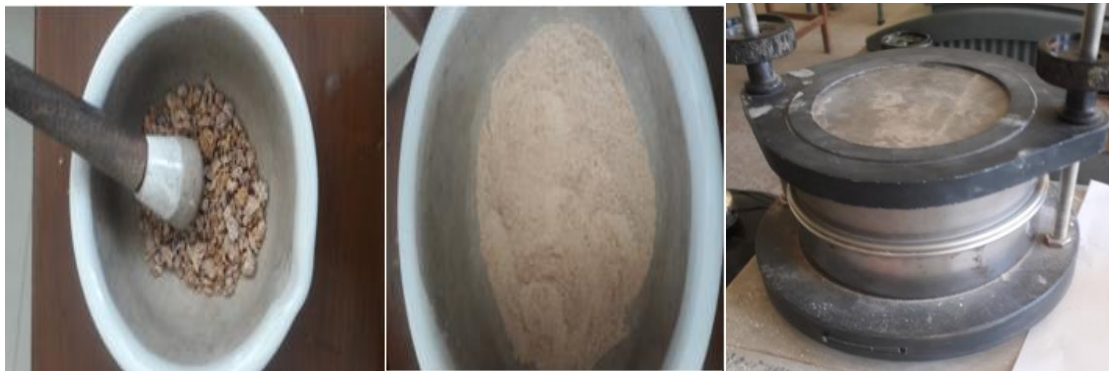
Figure 4: Powder of Enset passing through 150 \mu meter sieve size
