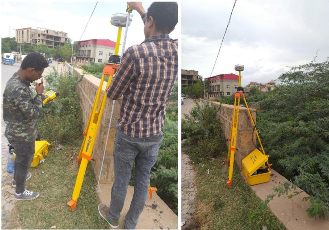
Figure 3.4: Checkpoint station of static GPS survey
