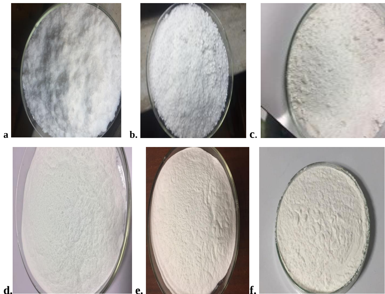
Fig.4. Cellulose extracted from corn husk(a), corn cob(b),lupine husk(c),and MCC from corn husk(d),corn cob(e),and lupine husk(f)
