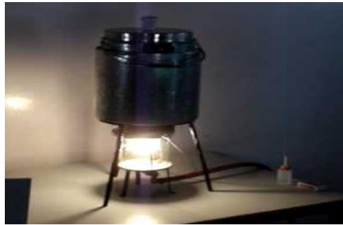
Figure 2-3 Ethanol heat stove [8]
