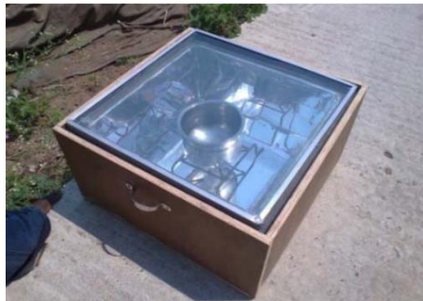
Figure 2-4 Box type solar cooker[9]
