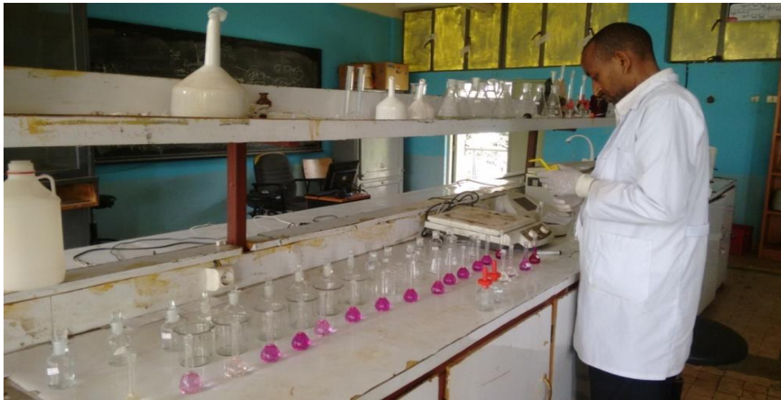
Appendix A.4: Adsorption process and determining Cr (VI) using diphenylcarbide method
