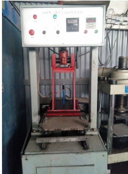
Figure 2.8 Kneading type compactor used in the rutting test apparatus. [31]
