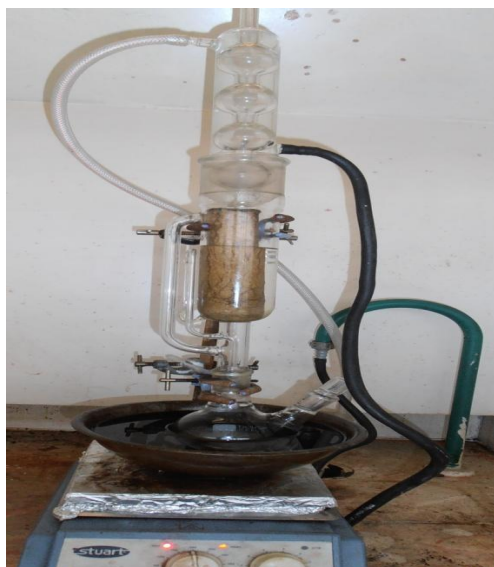
Figure 3.1: Set up of Soxhlet extraction
