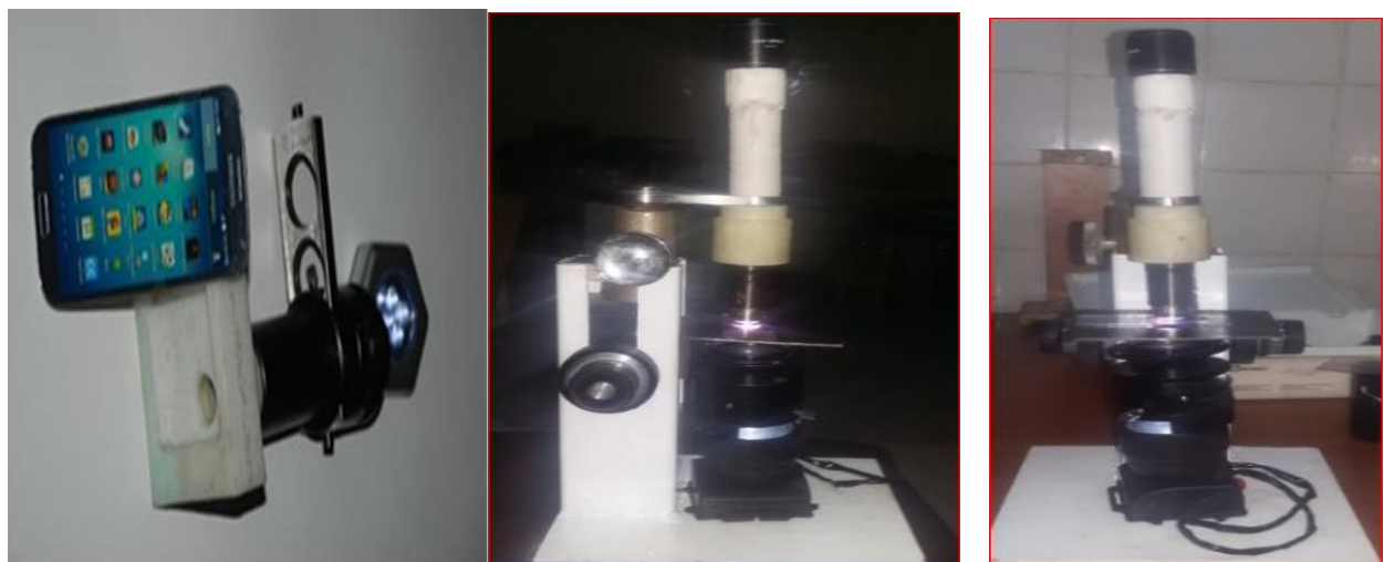
Figure 166: The first mobile phone microscope assembly result (left) and two views of the re-designed version of the mobile microscope (middle-right).
