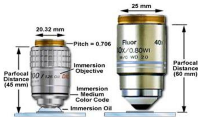
Figure 5: Parfocal length of the objective (45mm is standard).
