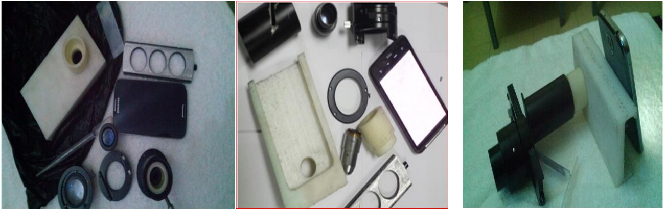
Figure 6: Basic parts of the proposed mobile microscope (left), another view of the basic parts of the mobile microscope (middle) and assembled version of the mobile microscope (right).
