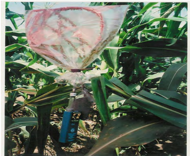
Figure 2.2 Pull headspace volatile collection of maize tassel.
