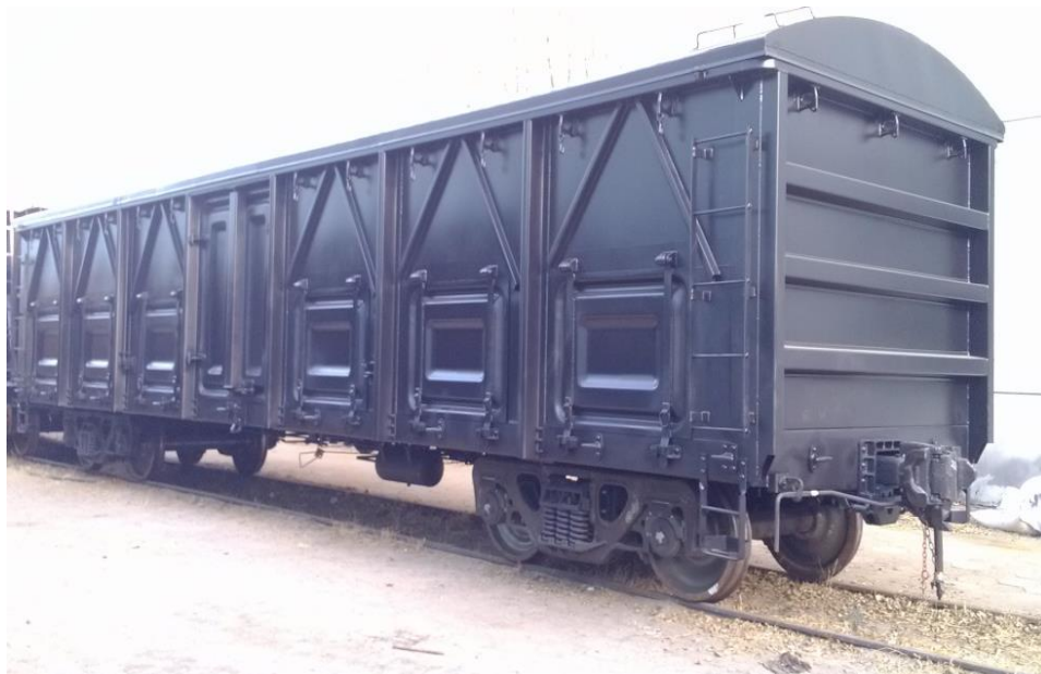
Figure 3. 2. Physical view of CW4 freight wagon used at Ethio-Djibouti line (Source: Ethio-Djibouti railway line project office)
