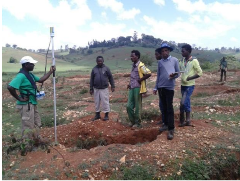
Figure 10 Data acquisition using ENVI PRO portable, proton-precession magnetometer in Biloya kebele where artisanal miners work following the river Biloya
