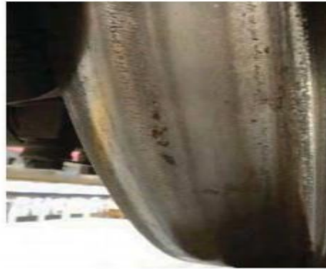
Figure 1.5. Wheel rolling contact fatigue [42]
