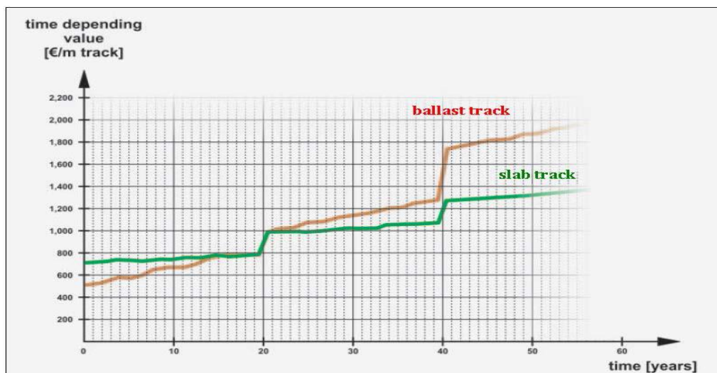
Figure 2-12: Time depending value, ballasted track and slab track (Rudolf & Dirk cited in Michas, 2012)
