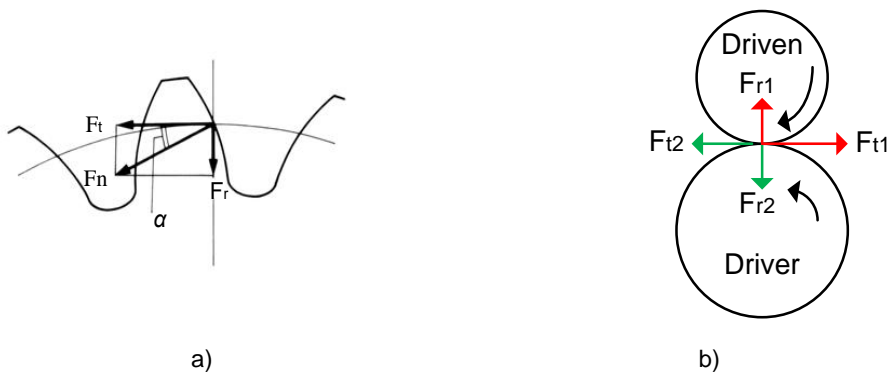
Figure 4.4 Forces acting on a spur gear mesh a) radial and tangential components in a single gear b) directions of forces acting on a spur gear mesh
