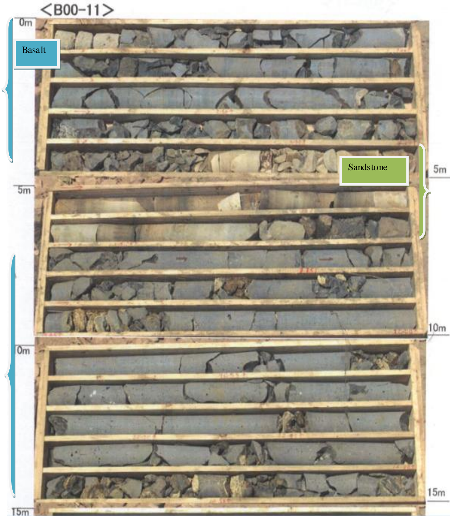
Figure 3-10 Core photographs for Bore Hole 11 at L/S00
