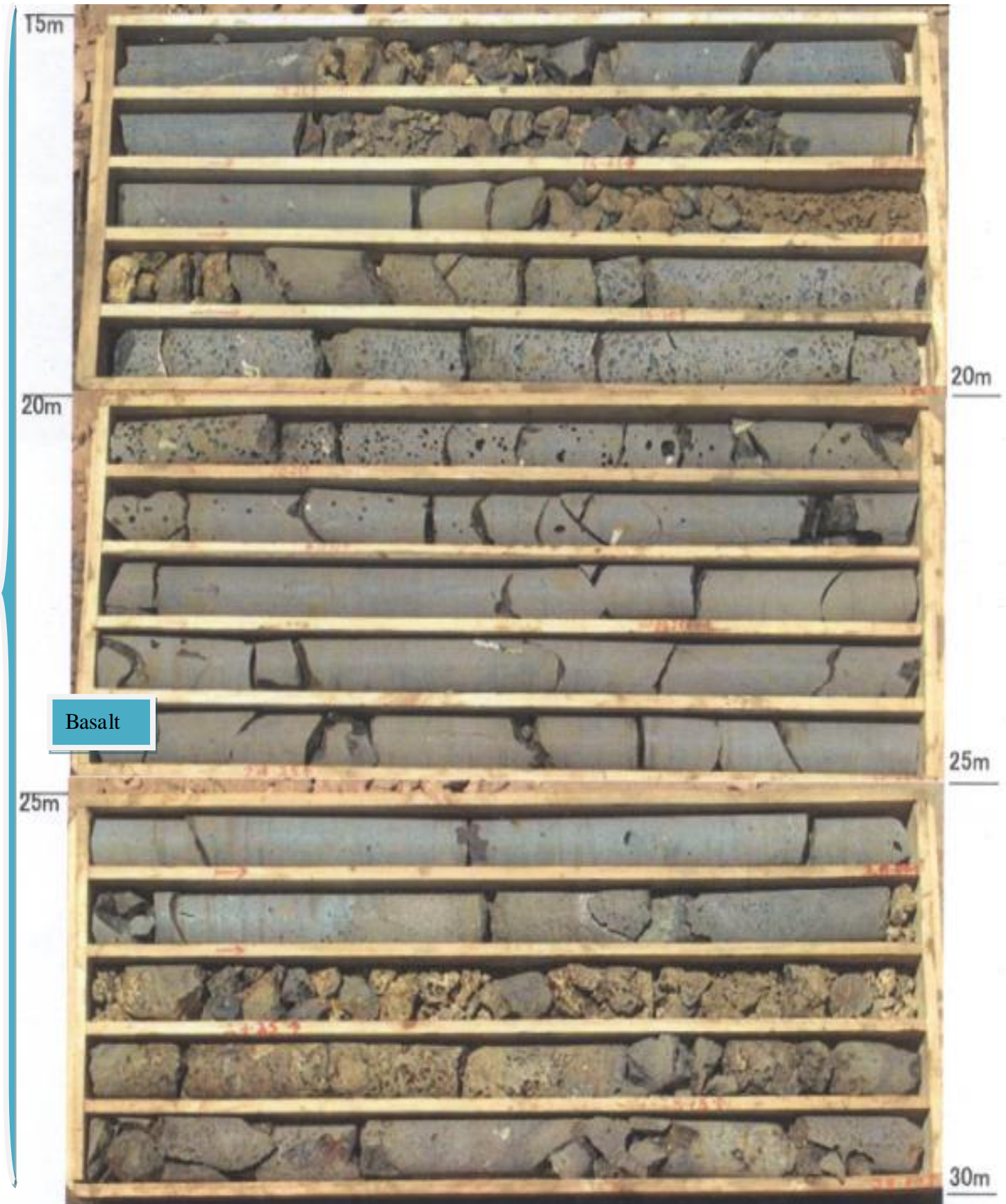
Figure 3-10 Core photographs for Bore Hole 11 at L/S00
