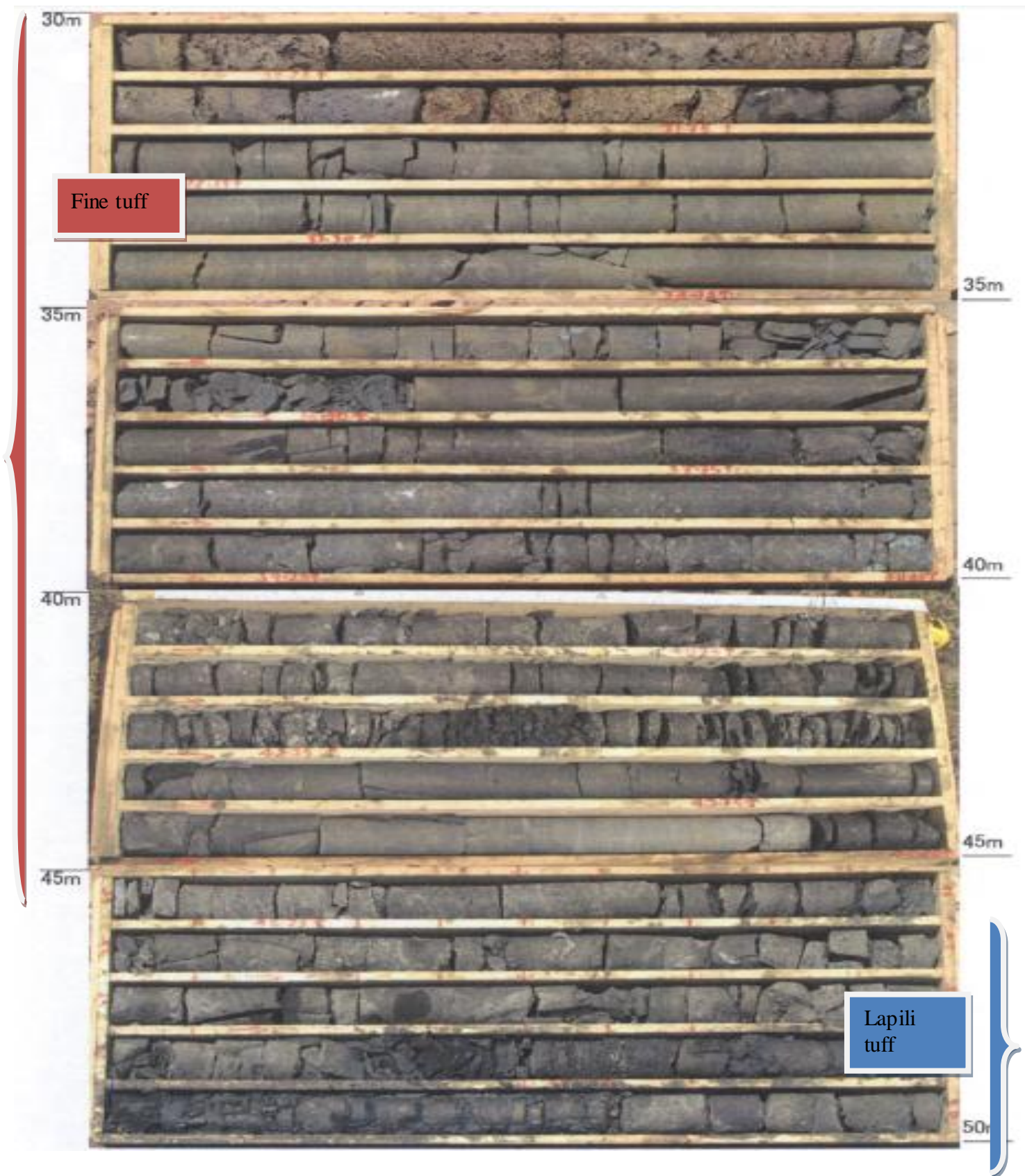
Figure 3-10 Core photographs for Bore Hole 11 at L/S00 (3)
