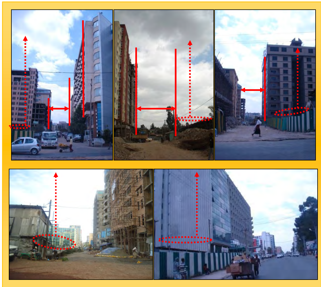
Pic - 3.5: Problems of the relationship of Setbacks, Streets width and building height.
