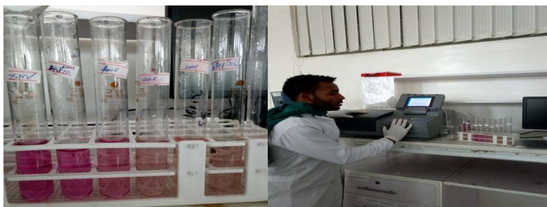
Figure 6: Standard solution and measurement of its absorbance using UV-spectrophotometer
