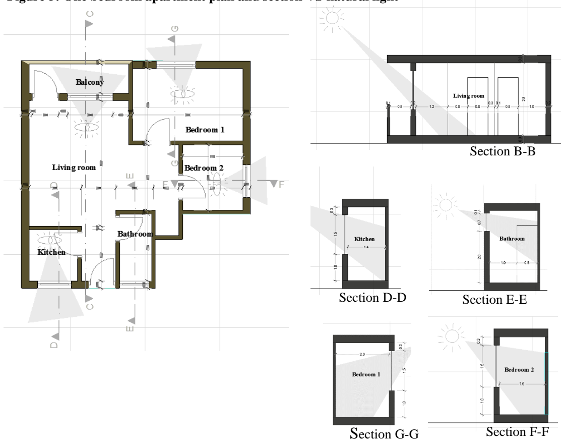
Figure 6: Two-bedroom apartment plan and section VS natural light
