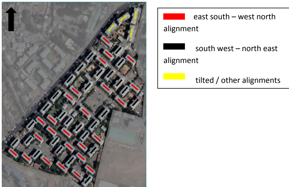
Figure 4: Alignments of blocks Vs sun path
