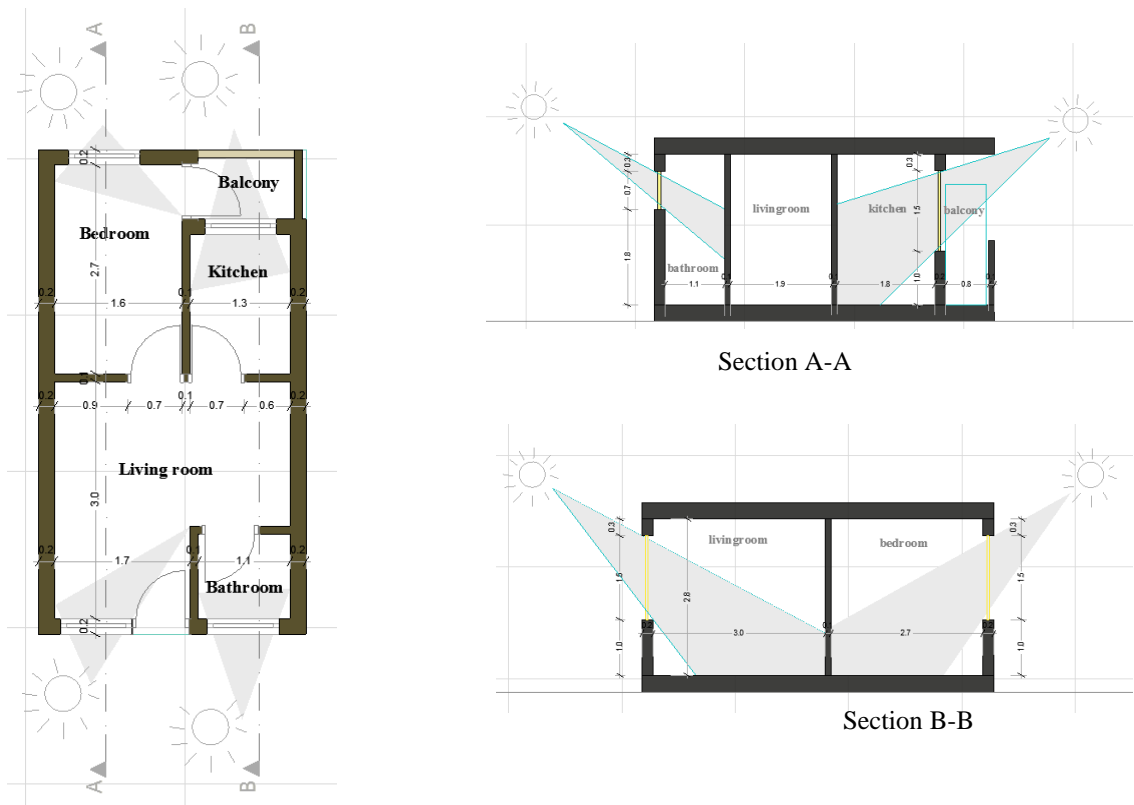
Figure 5: One bedroom apartment plan and section VS natural light
