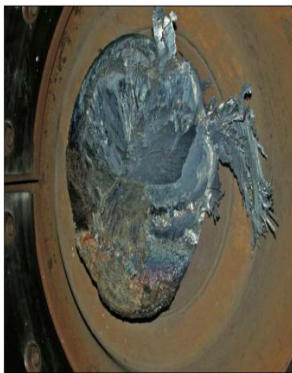
Fig 2. 7: Fractured surface of an axle [13]
