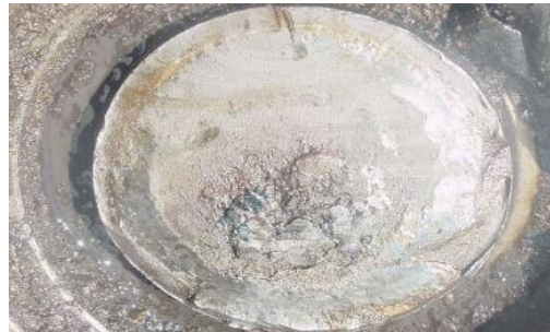
Fig 1. 1: Broken tank wagon axle from a severe derailment [3]
