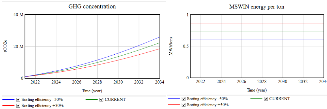
Fig 4.3 sensitivity of sorting efficiency on waste calorific level, produced MSW incineration energy and Total GHG concentration.
