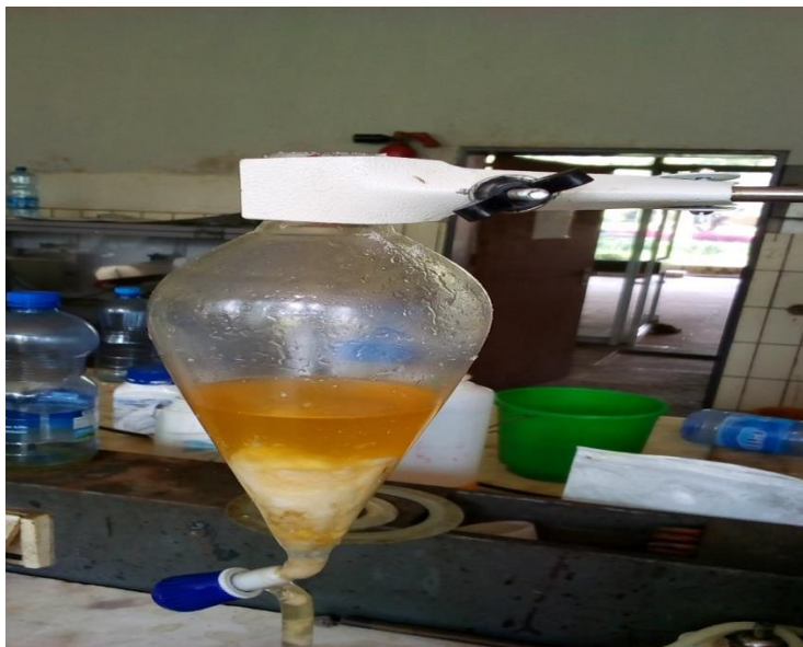
Figure 3-5: crude oil washing and neutralization
