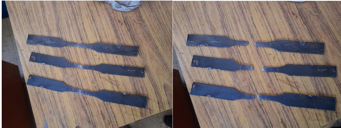
Fig 3. 2 Tensile test on steel tubes
