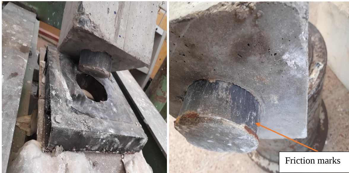
Fig 5. 4 Friction resistance of steel tube at the interfaces
