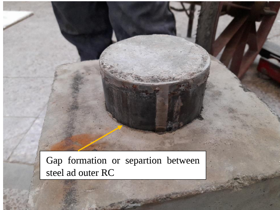
Fig 5. 17 Gap formation on the free end of the interfaces
