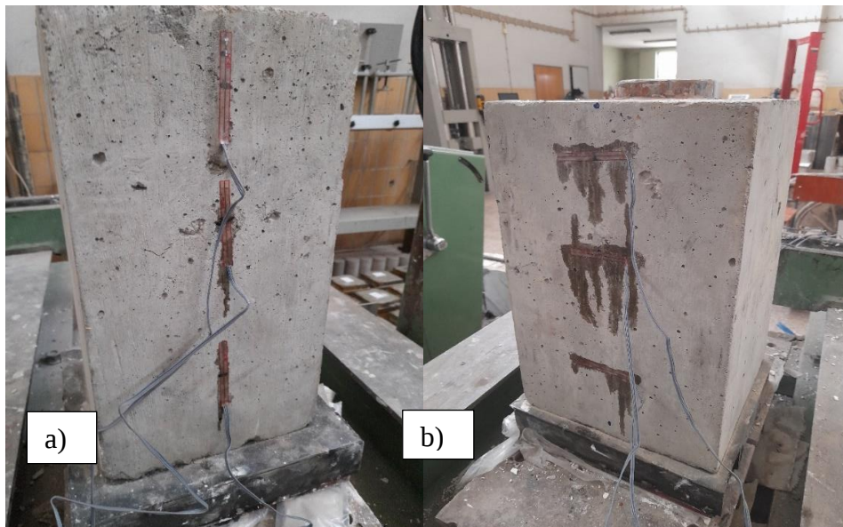
Fig 3. 8 strain gauges arrangement a) Longitudinal strain gauge b) transverse strain gauge
