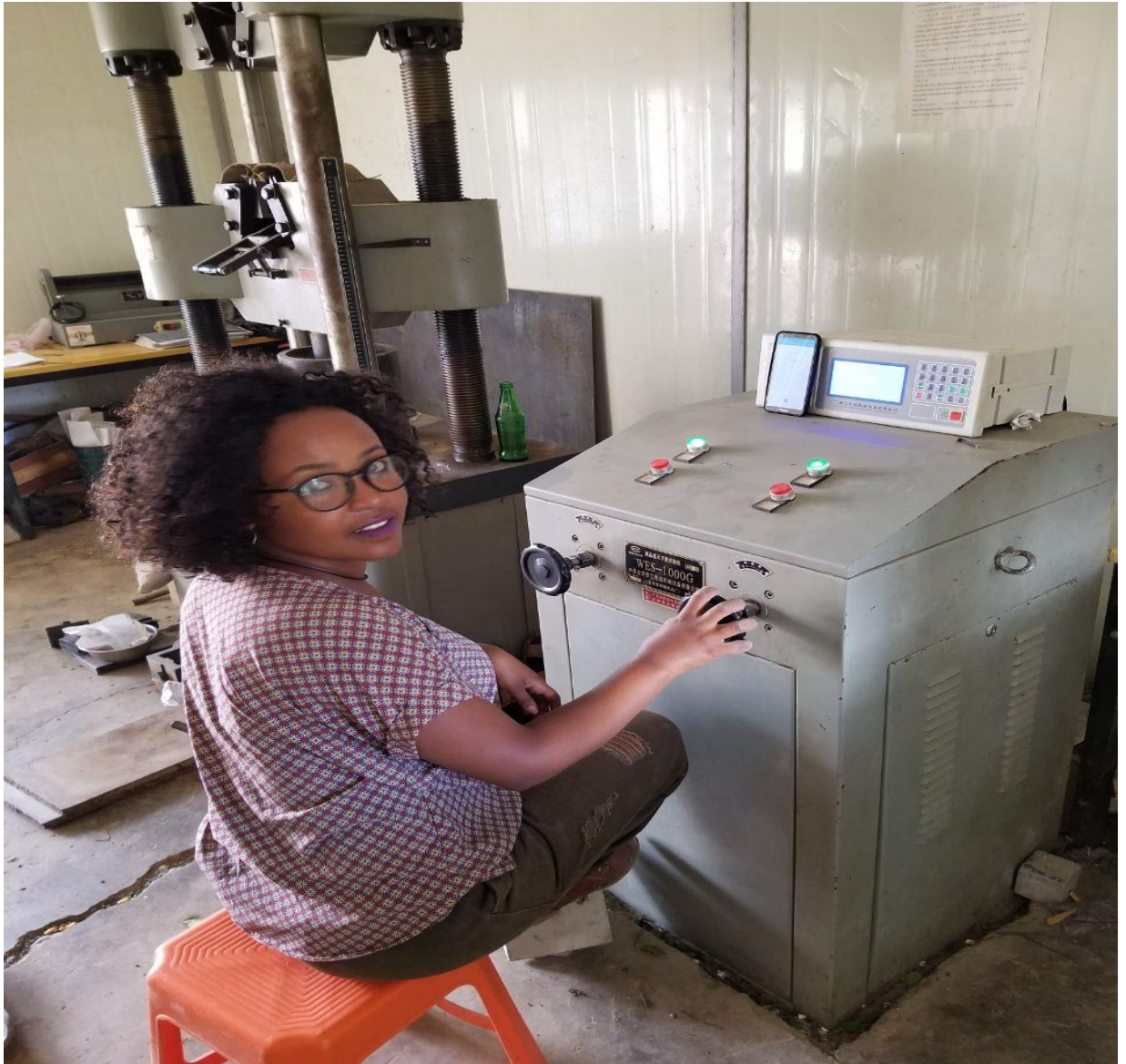
Figure 5-5 Crushing Value Test for Ballast
