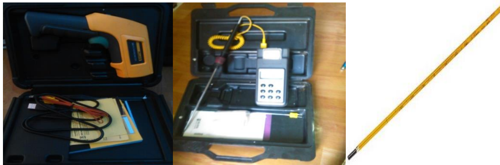
Figure 3.1: Temperature measuring instruments (a) Infrared thermometer (b) K- type thermocouple (c) glass thermometer
