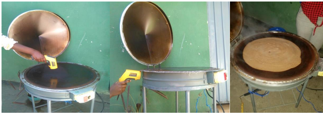
Figure 3.2: Actual picture during experimental investigation (a) & (b) pictures of experimental set up (c). Injera texture
