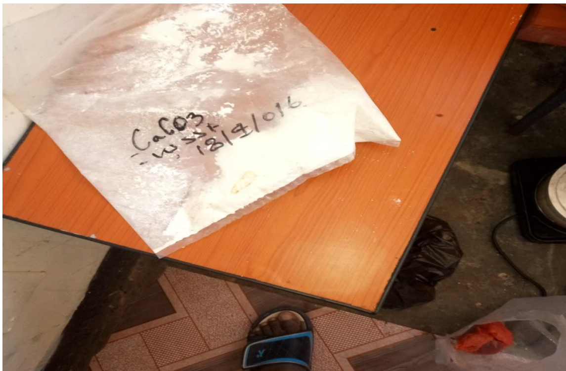
Appendix Photo 6. The CaCO 3 used to precipitate the phosphate
