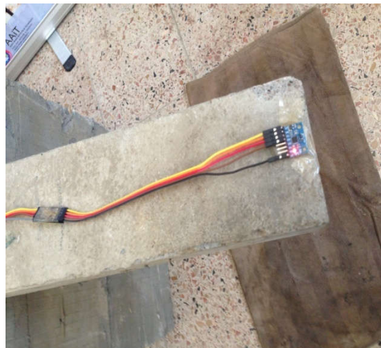
Two Set up of MPU6050 sensor (above and below the specimens)
