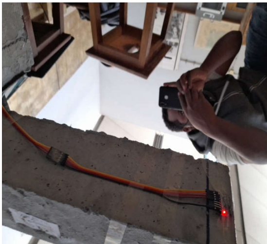
Two Set up of MPU6050 sensor (above and below the specimens)
