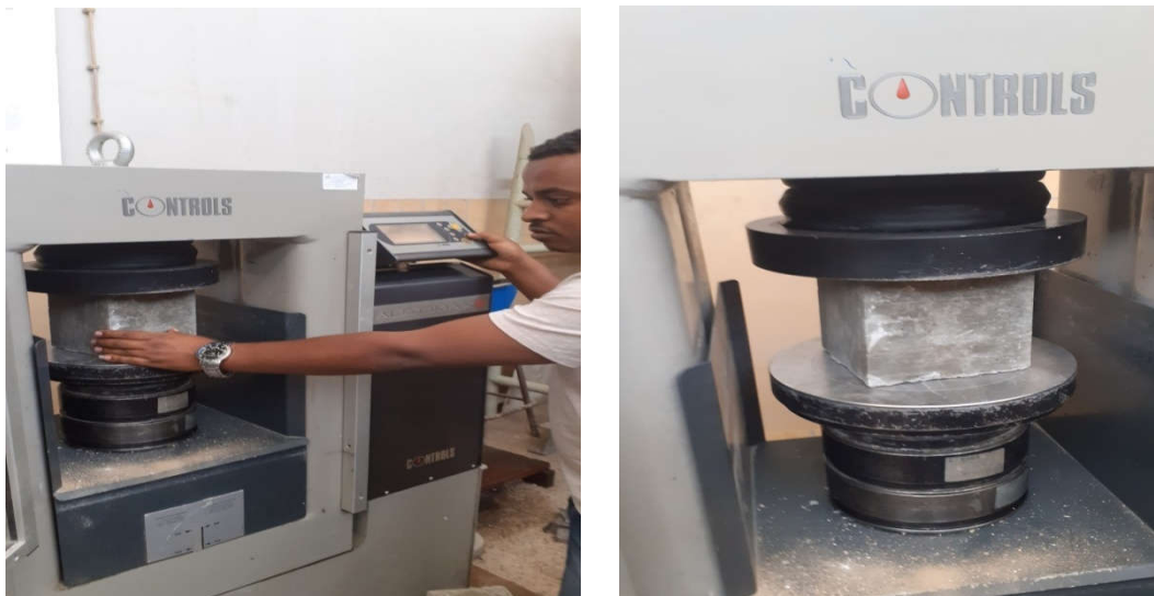
Figure 3.5: Compressive strength test set up for cubes
