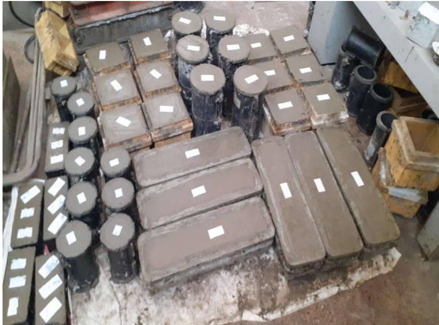
Sample of Flexural specimens, cylinders and cubes contains waste tyre rubber
