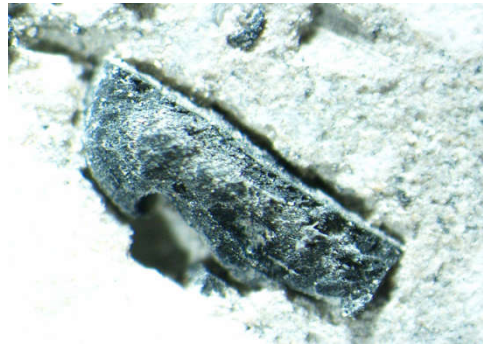
Figure 2.1 Bonding between cement paste and rubber particle.( Dubravka et al. 2011)
