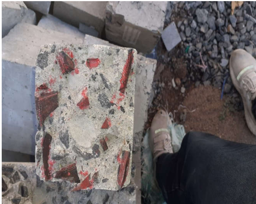
Rubber particles distribution in concrete matrix after failure during compressive loading
