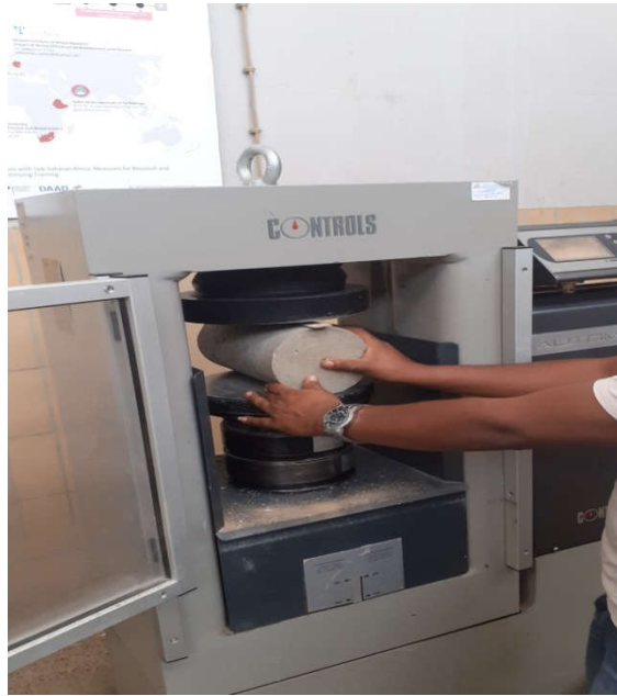
Figure 3.7: Split tensile test set up for cylinders
