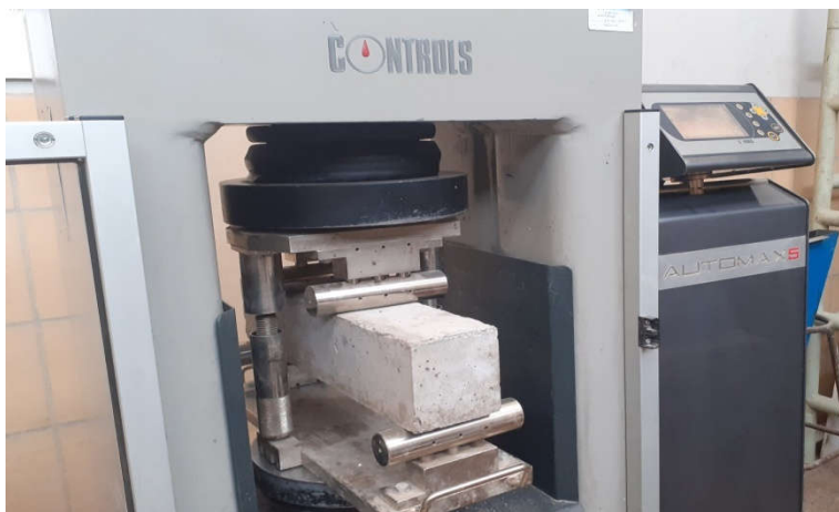
Figure 3.9: Flexural strength test set up for prisms by third point loading using UTM
