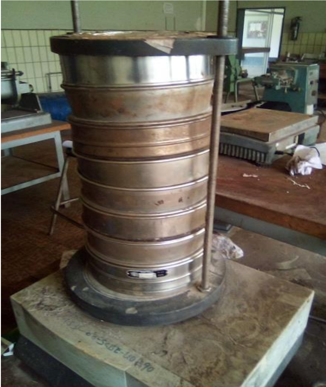
Figure 3.4. ASTM standard sieve shaker at AAiT laboratory
