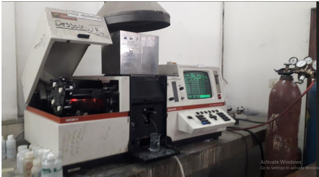
Figure 3.6. AAS calibrated for chemical analysis
