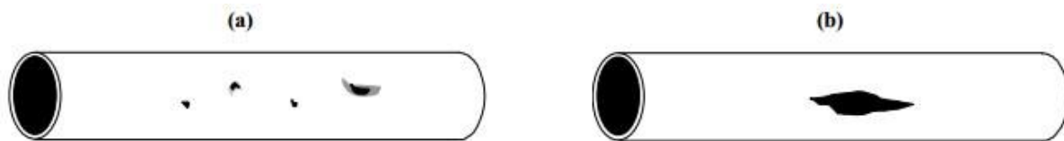
Figure 2.5 (a) corrosion pitting and (b) blow-out hole
