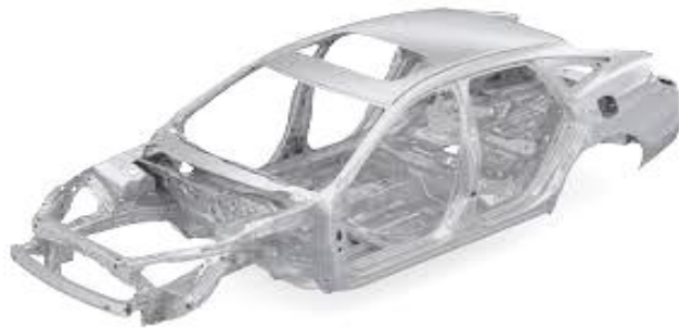
Figure 3 typical passenger's car of monocoque structure
