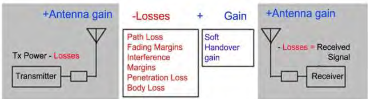
Figure 1 A simplified block diagram of the link budget calculations
