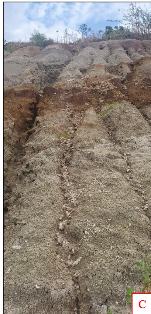
Figure 4-8: A & B) Formations of rills and gullies on the surface of slope C) Crack and fissures on the surface of slope soil
