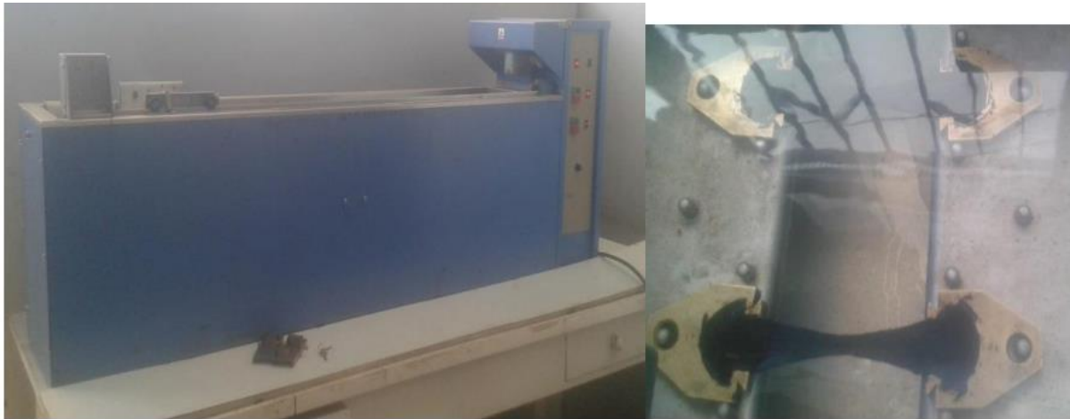
Figure 9: Ductility test setup
