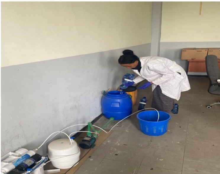
Annex 4: Filling Feed water tank of RO Filtration
