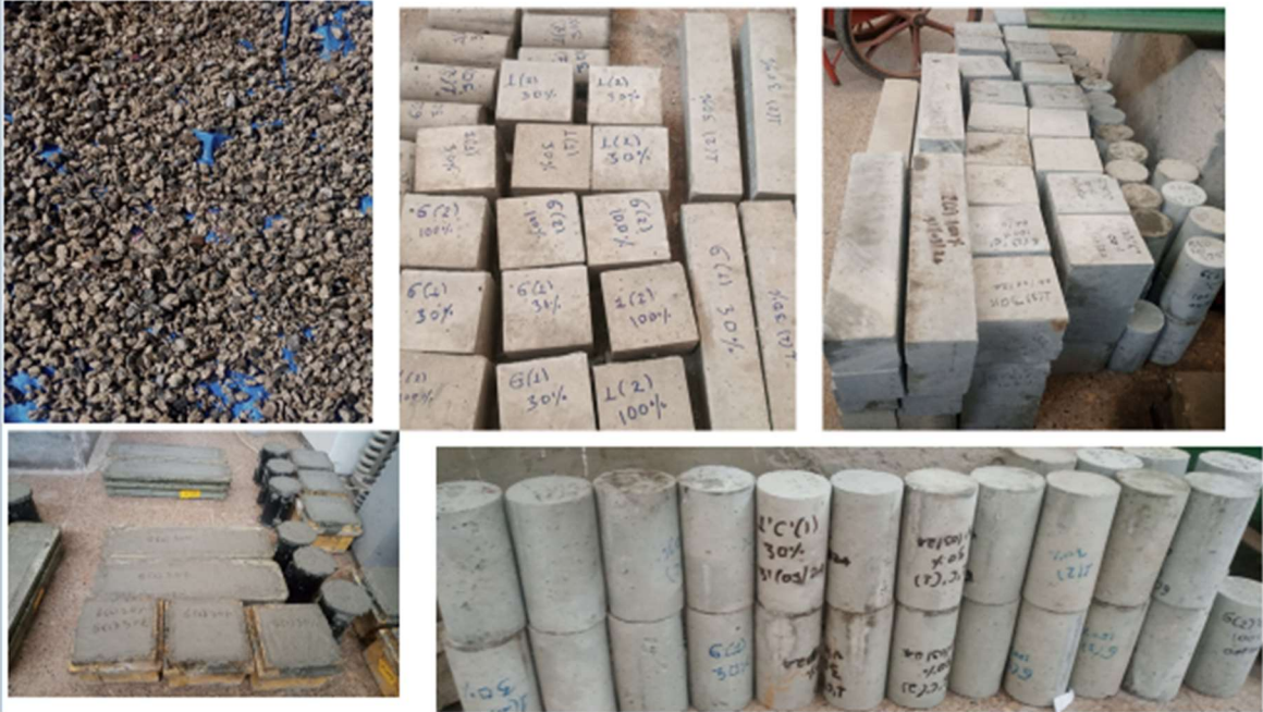
ARCA @SSD, Casting, and cured samples ready for strength test
