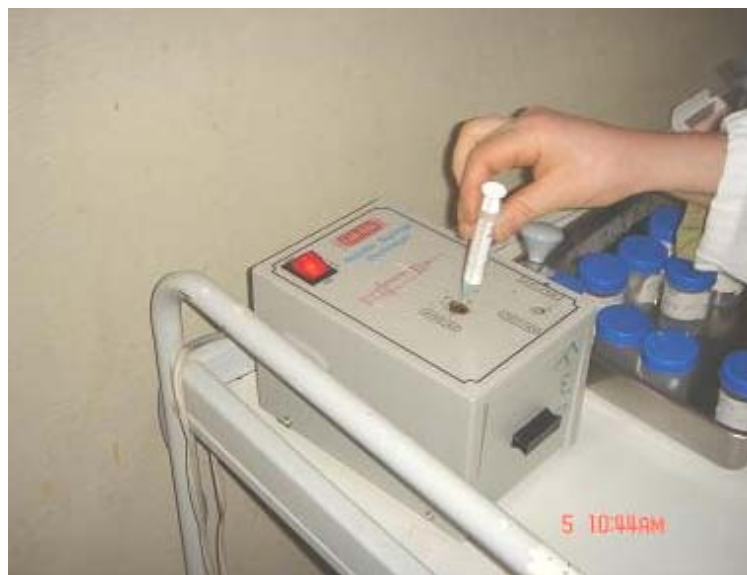
Figure 4.8 On-site needle incinerator
