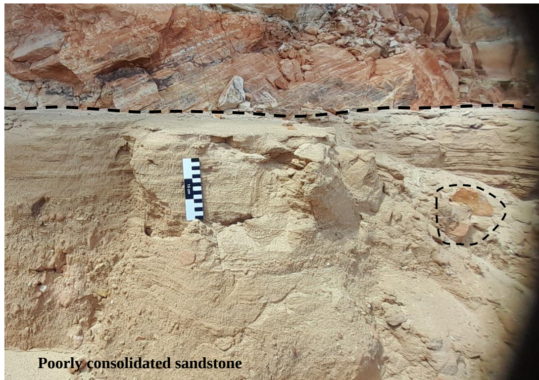
Figure 5. 3 Loosely-consolidated sandstone with very thin lamination, the black circles show the cobble size.
