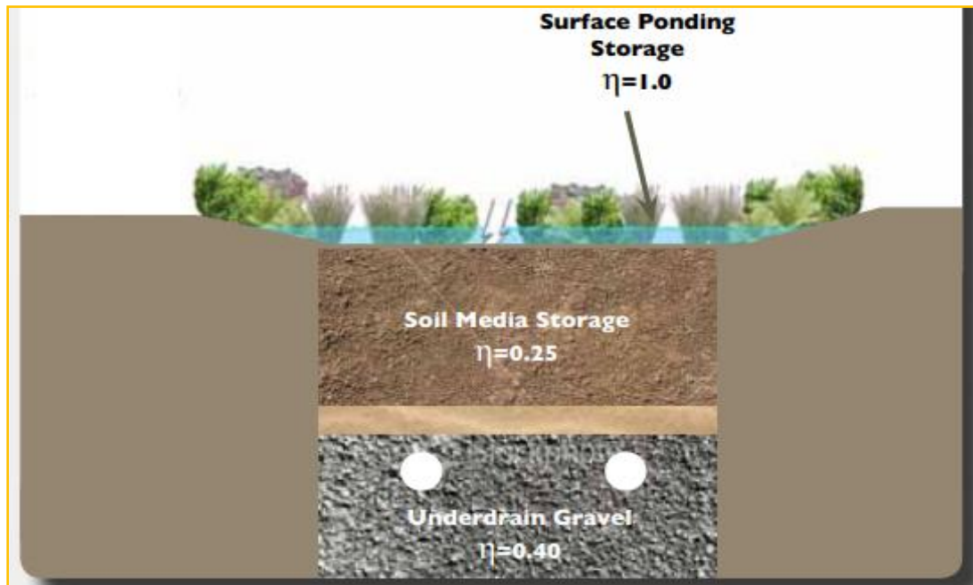
Figure 3-7. Typical Bio retention Section with Porosity ( n ) Values for Volume Computations (Source: West Virginia storm Water Management and design guidance Manual).
