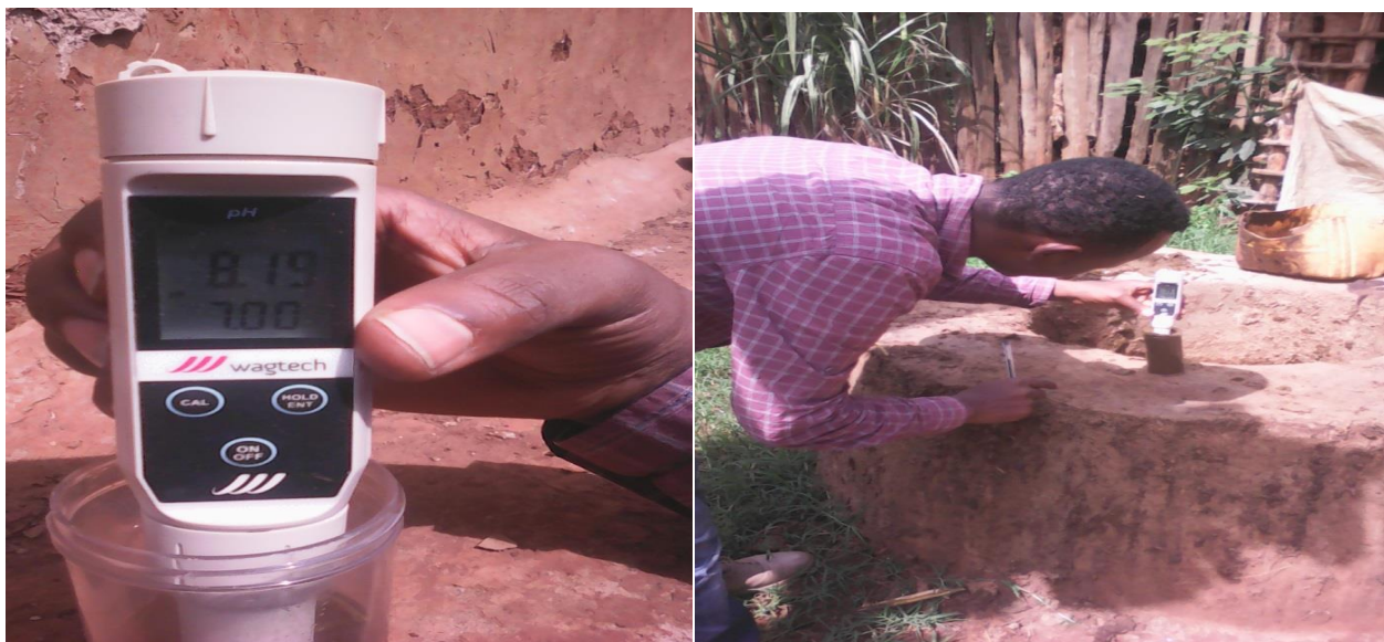
Figure 3.2: Portable PH and Temperature measuring instrument and analysis (Source field measurement of, 2018)
