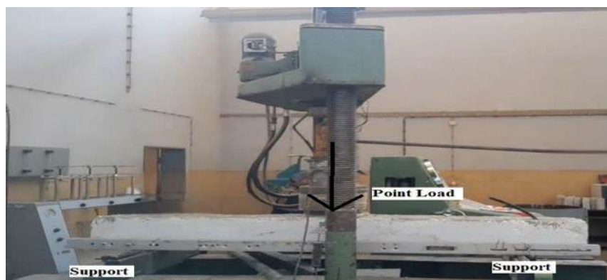
Figure 3.8: Testing Machine Setup
