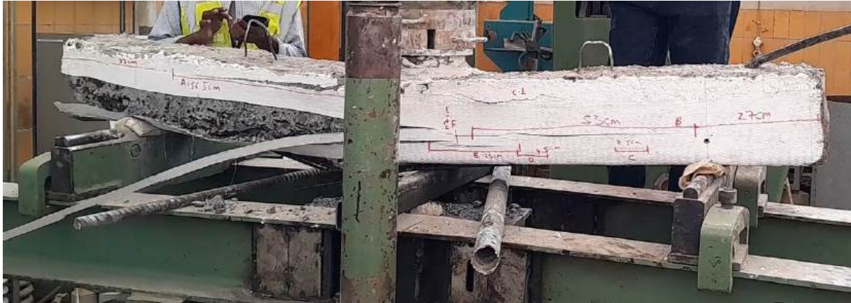
Figure A.24: G3B-22 Right Side Tear & Delamination
