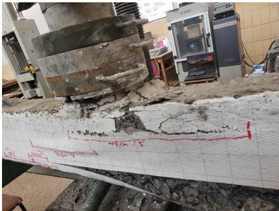
Figure A.9: Concrete Crushing and Spalling at top of the beam
