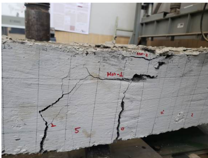
Figure A.13: Right Side Failure State of G3B-30
