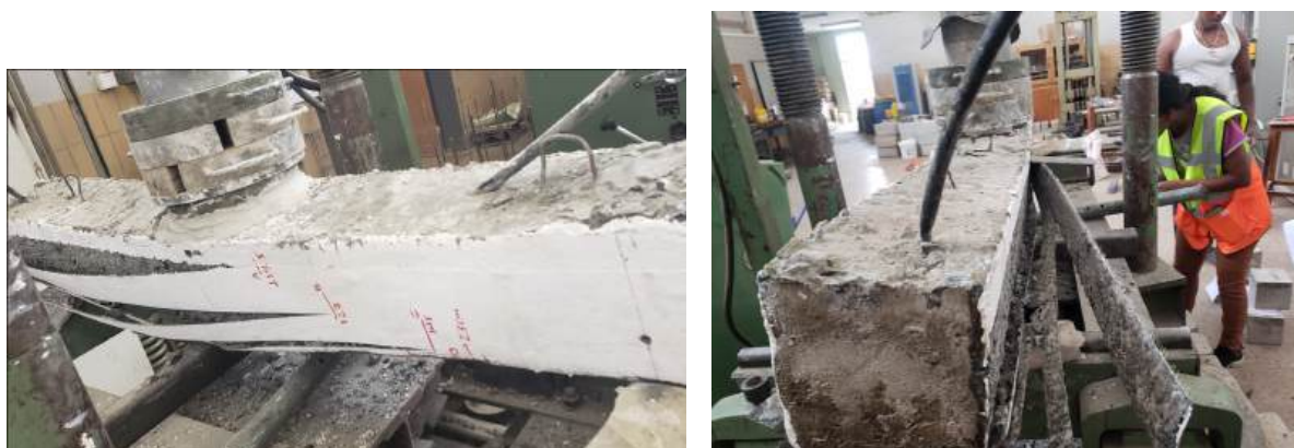
Figure A.11: G2B-12 Left Side CFRP Tear & Delamination
