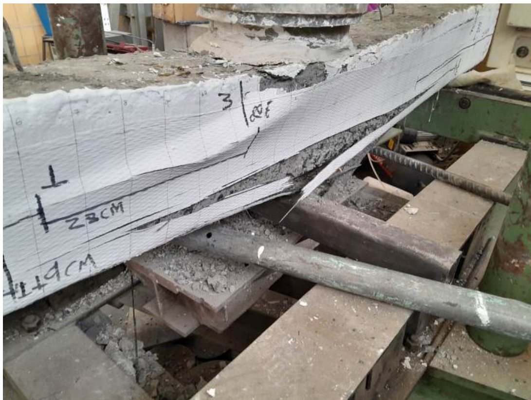
Figure A.25: G3B-22 Left Side Tear & Delamination
