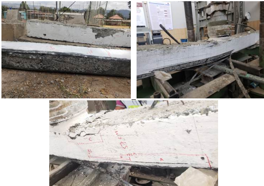
Figure A.7: G2B-11 After Testing Bottom, Right & Left Side CFRP Tear & Delamination (right, left & bottom)
