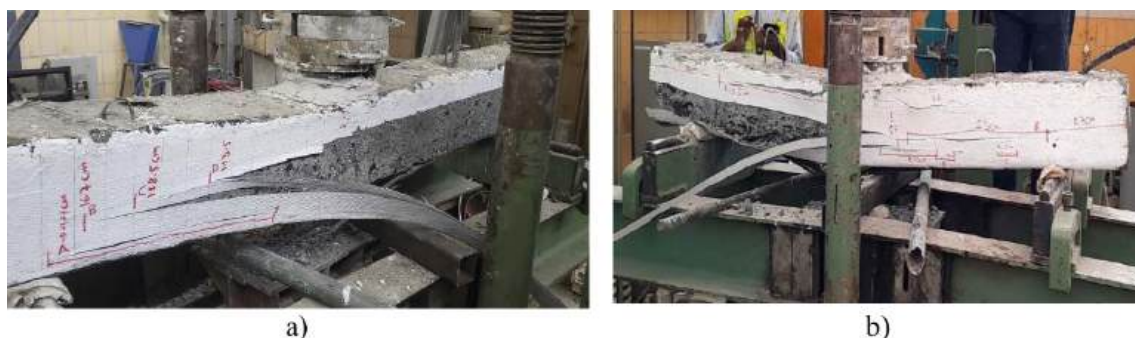
Figure 4.6: Rupture and delamination of a) G3B-21 and b) G3B-22
