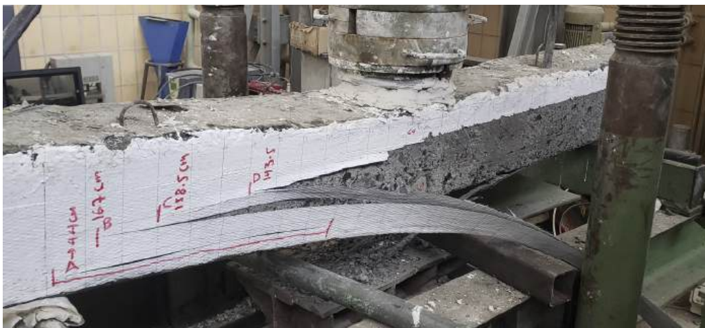
Figure A.20: G3B-21 Right Side Tear & Delamination
