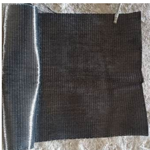
Figure 3.3: CFRP Sheet Used
