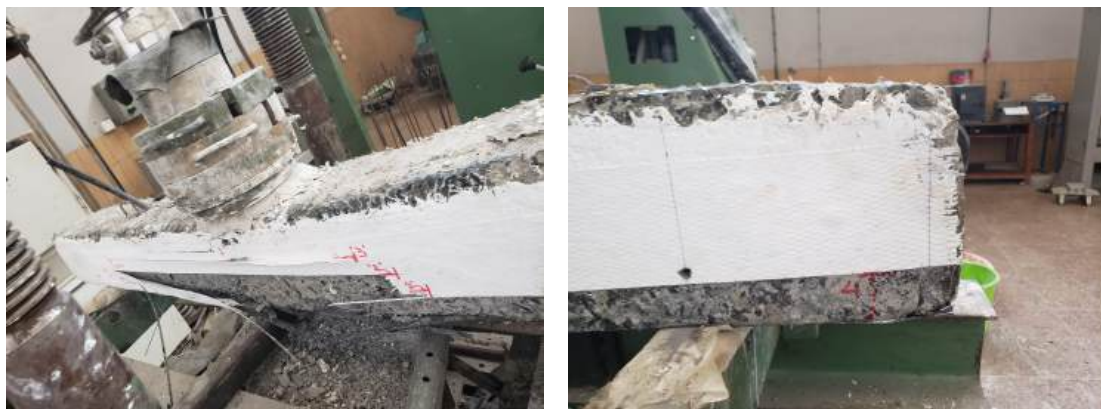
Figure A.21: G3B-21 Left Side Tear & Delamination
