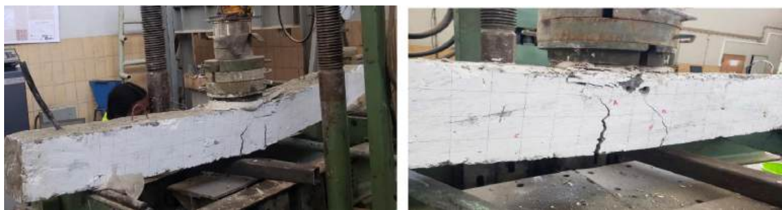
Figure 4.1: Failure of G2B-20
