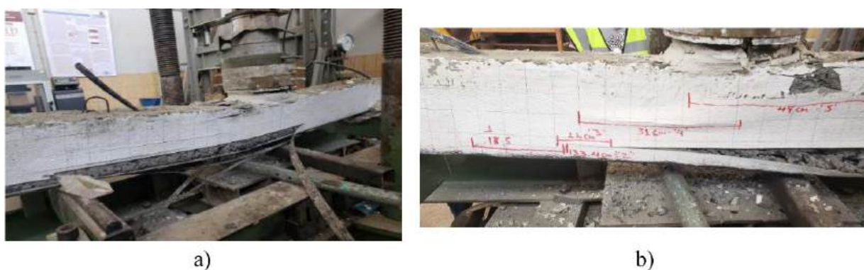
Figure 4.3: a) deformed shape of G2B-11 and b) rupture and delamination of CFRP, G2B-12
