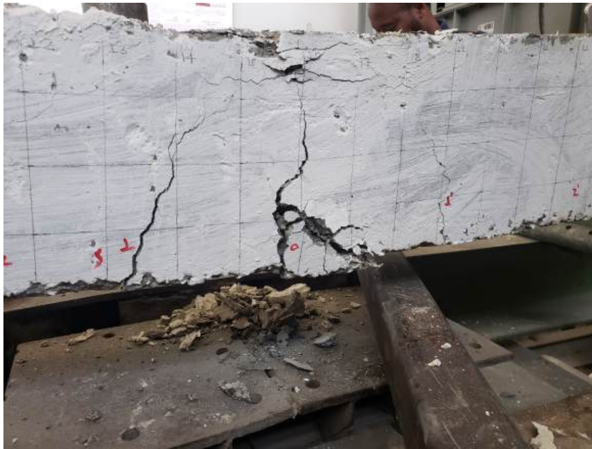
Figure A.17: G3B-20 Flexural Crack and Concrete Crushing (Top & Bottom Center)
