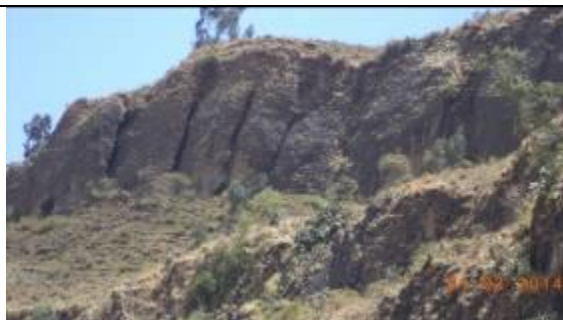
Fig 4.9a. Open Joints at the top of the cliff with orientation strike N 20°-30° E and dip more or less vertical.
