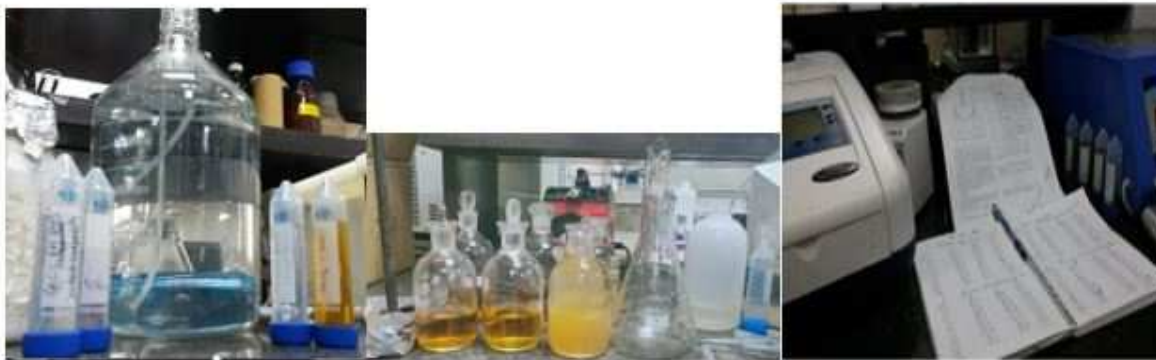
Figure 40 Biological oxygen demand buffer preparation, titration and color analysis
