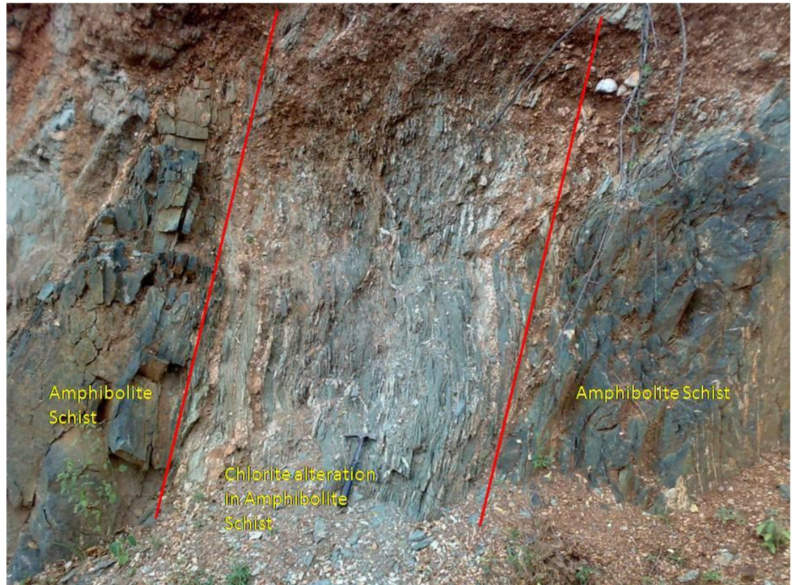
Photo 7. Photo taken in trench 295, showing 1.5 m length highly mylonitized and hydrothermally altered part of chlorite amphibole schist
