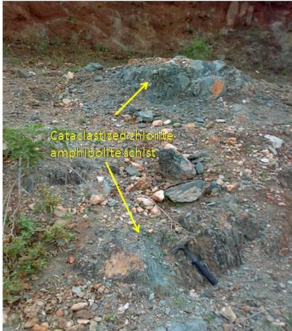
Photo 30. The picture taken around borehole number 212 in North Okote shows cataclastized chlorite amphibolite schist
