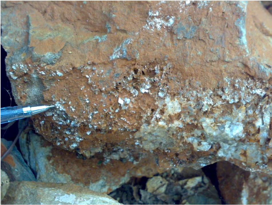
Photo 15. Sericite minerals inside the fracture plane that is found closer to the ore body
