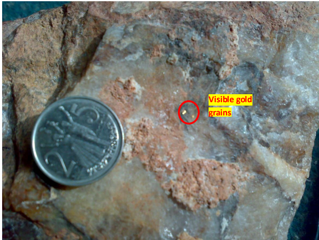
Photo 18. Hand specimen from Okote, shows a quartz carbonate vein (Quartz vein 2) with visible gold grain
