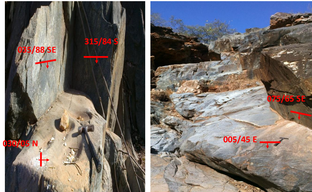
Photo 27. Shows a picture taken in a river outcrop of chlorite amphibolite schist with strike and dip amount of joint systems in central part of the study area. Scale geological hammer
