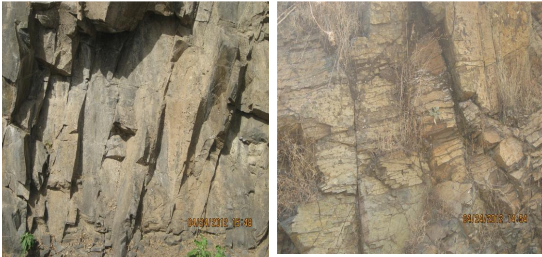
Figure 5.12. Joints in the Upper Basalt aquifer.
