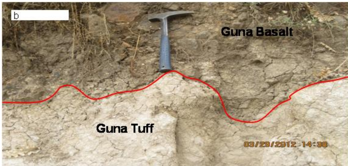
Figure 3.8. Contact between Guna Tuff and a) Upper Basalt and b) Guna Basalt
