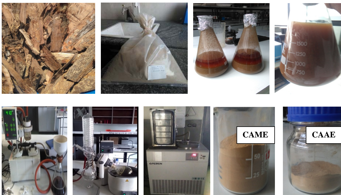
Figure 3. 1: Photos of collected stem bark sample of C. africana , powdered sample, methanol and aqueous extracts, filtering of extracts, concentrating extracts and their yields.
