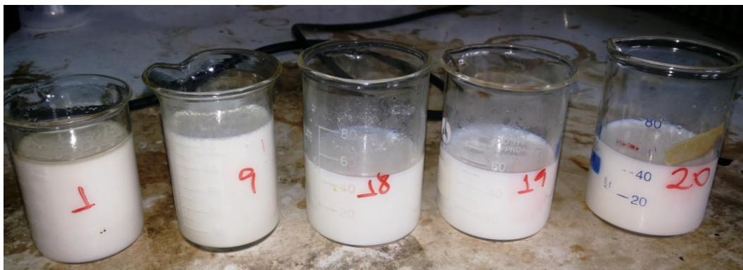
Figure 4.11: Ten percent emulsion formed by sulphited fatliquor
