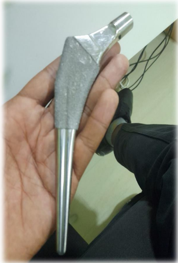
Figure 10:FEMUR STEM: is a component of a total hip replacement, which is a surgical procedure that replaces a damaged or arthritic hip joint with an artificial joint. The femur stem is the portion of the implant that is inserted into the femur bone. Material for femur stem: Ti-6Al-4V means It is comprised of 90% titanium, 6% aluminum and 4% vanadium. Taperlock complete primary femoral porous coated stem. 8x136mm standard offset 12/14 taper for cementless use
