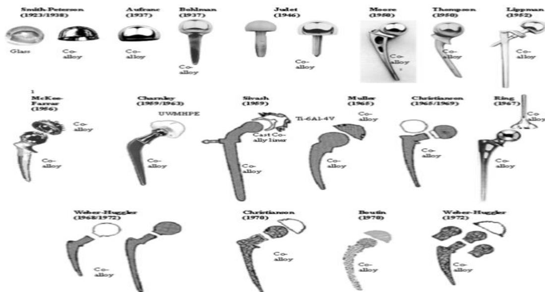
Figure 3: The history of the development of the regular straight stem in hip arthroplasty [22].
