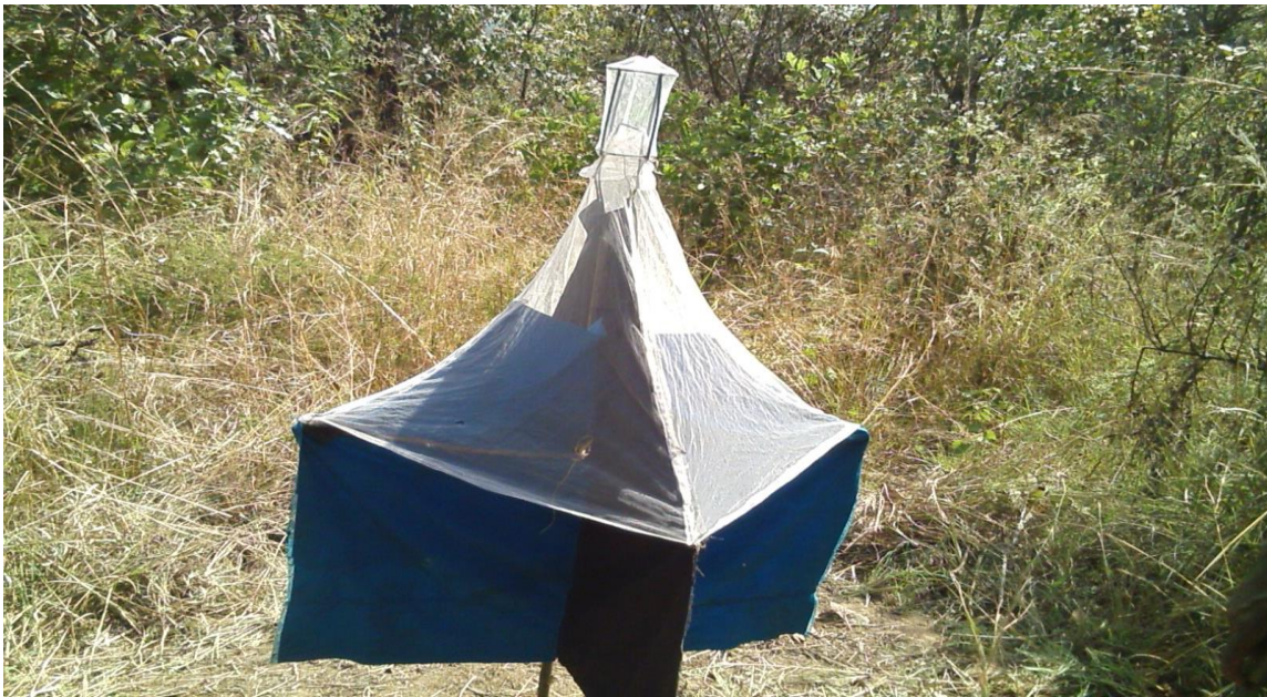
Figure 3: Monoconical trap deployed for entomological study, Giray Sonka, Gidami District, Kellem Wollega Zone, Oromia Regional State, Ethiopia
