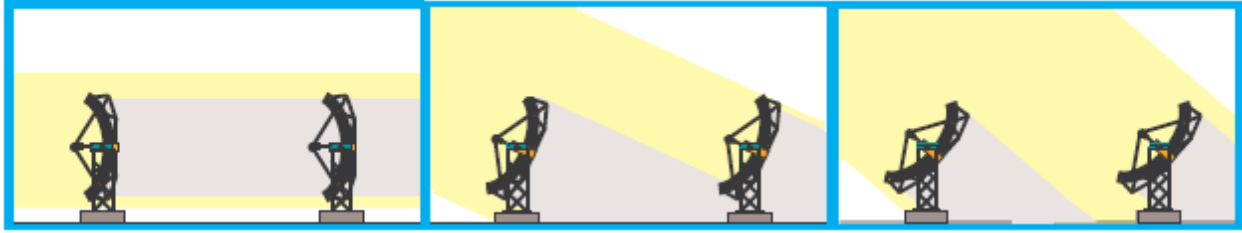
Figure 2-10 Collector tracking through morning, showing digression of collector shading as the day progresses [22]
